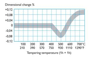
Note: The dimensional changes in hardening and tempering should be added.
