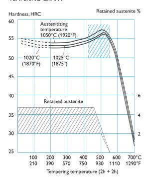
Tempering within the range 425–550°C (800–1020°F) is not normally recommended due to the reduction in toughness properties.
