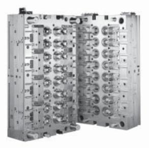
Uddeholm RoyAlloy is the preferred steel of choice of many mould makers and end users. Uddeholm RoyAlloy provides enhanced machinability, improved dimensional stability and superior surface finishes compared with AISI 420F/W-Nr. 1.2085 type of steel.
