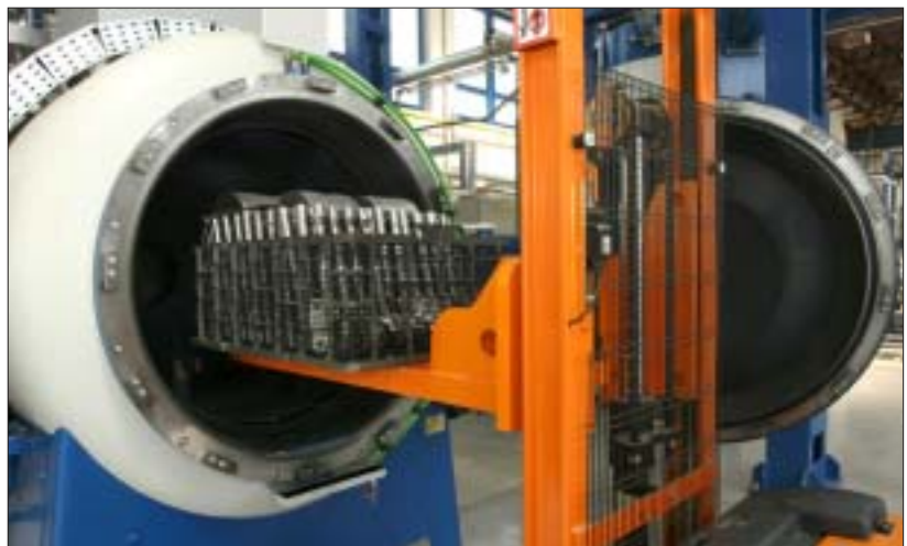
Charging operation. Photo: Böhler Uddeholm Czech Republic.
