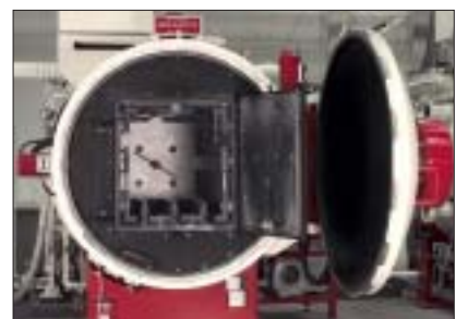
Hot zone with graphite insulation. Photo: Schmetz GmbH Vacuum Furnaces, Germany.
