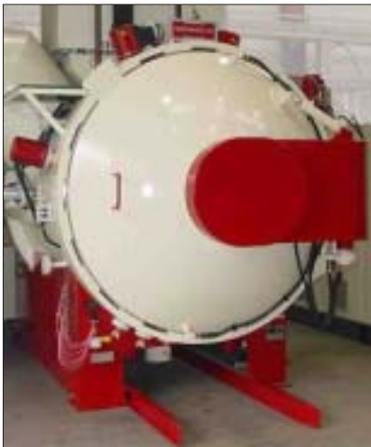
Vacuum furnace. Photo: Schmetz GmbH Vacuum Furnaces, Germany.
